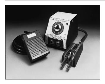
The ease and simplicity of operation of the Thermal Wire Stripper make it ideal for most strain gage leadwire stripping. The variable heat control allows stripping of all thermoplastic insulations, including Teflon<sup>®</sup>, in sizes No. 18 to No. 36 AWG [1 to 0.1mm diameter]. The foot switch and tweezer handpiece give excellent operator control over the stripping operation. Includes power unit and foot switch, both with 3-wire NEMA plugs, and tweezer handpiece.
