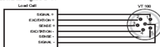
Figure 2-5: 6-Wire Load Cell Application
