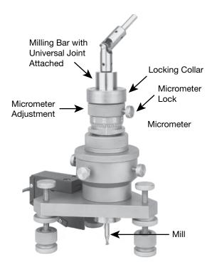
Conventional slow-speed milling may be satisfactory on some mild steels and aluminum alloys. But high-speed drilling is generally the most convenient and practical method for introducing the hole in all test materials. (When residual stresses are to be measured on materials such as stainless steels, nickel-based alloys, etc., ultra high-speed drilling techniques are preferred.) For this purpose, a high-speed air-turbine assembly, along with a supply of tungsten carbide-tipped cutters [ten
