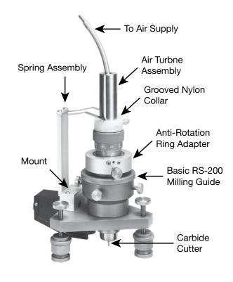
A micrometer depth set attachment, available in English or metric units, is provided with each milling guide assembly. This device is used for incremental drilling when information on the variation of residual-stress-with-depth is desired.
