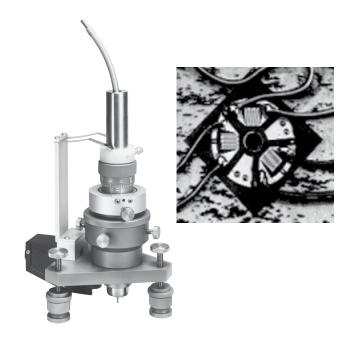
steel housing with eyepiece, reticle, and objective lens, permits alignment to within 0.0015 in (0.038 mm) of the gage center. The microscope is also used to measure the diameter of the hole after it is drilled. An illuminator attaches to the base of the guide to aid in the optical alignment procedure.
