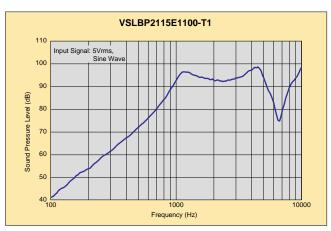
Measurement Condition of Sound Pressure Level: Input Signal: 5.0Vrms, Sine Wave, at 100mm Back Cavity: VSLBP1913E1400-T1 (VSLBF1913E1400-T1)=0.7cc, VSLBP2115E1100-T1=1.0cc
