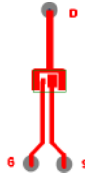
⑩ Mounted on minimum footprint full size board with metalized back and with small clip heatsink (still air)
