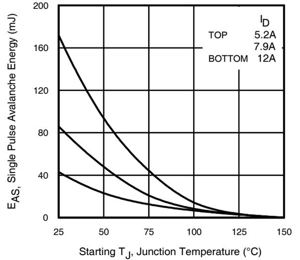
**Fig 13.** Maximum Avalanche Energy Vs. Drain Current
