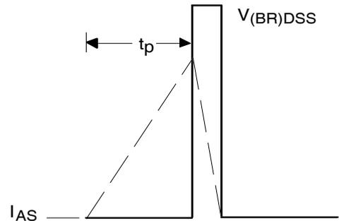
**Fig 14b.** Unclamped Inductive Waveforms
