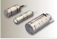
Vishay Systems offers a unique series of load beams for use as axles, pins, and shafts. These cells replace "dead" shafts in bogies, pulleys, and coupling devices, thereby providing live force measurement for crane scales, aircraft/ ship wheel bogies, push-pull systems, and other onboard devices.
