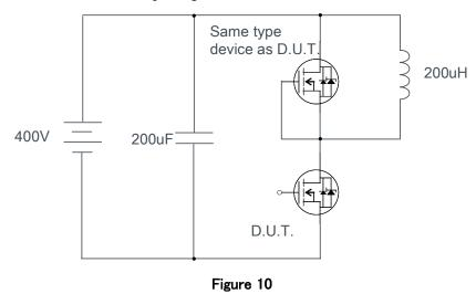
The turn-on switching rate of SiC-MOSFET is several tens of nanoseconds, which is equivalent to that of Si-IGBT and Si-MOSFET. However, inductive load switching causes a recovery current from commutation to the upper arm diodes to pass through the lower arm.
