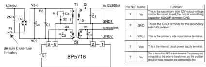
For actual usage, Please kindly evaluate and confirm our part mounted in your product, Especially, Please make sure to confirm whether the load current exceed Max. rated current by using the current probe.
