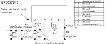
For actual usage, Please kindly evaluate and confirm our part mounted in your product, Especially, Please make sure to confirm whether the load current exceed Max. rated current by using the current probe.
