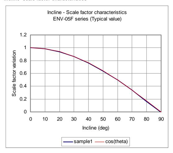
The scale factor change when installing the sensor inclined to rotation axis. The scale factor variation obeys the following equation.
