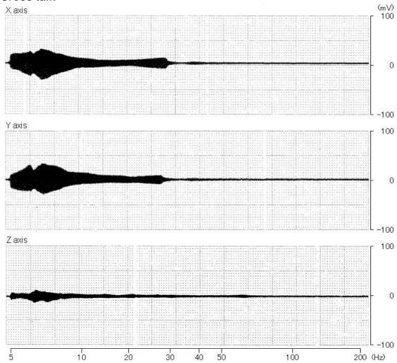
The static output under the vibration of which frequency is 5~200Hz and of which acceleration is 1G.
