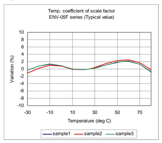
The scale factor change over operation temperature.
