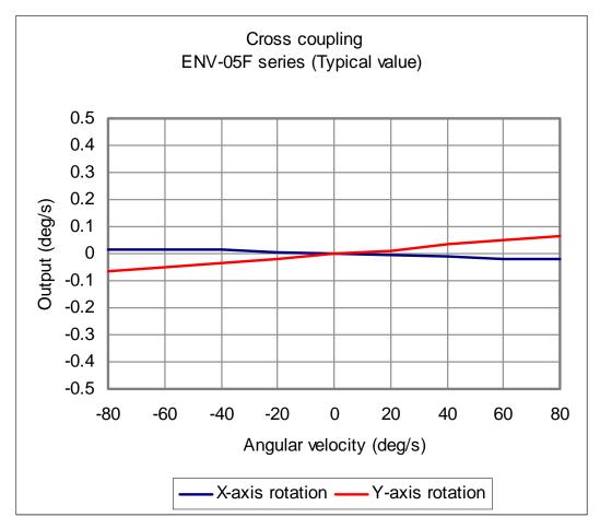
The cross coupling signifies output error applied unnecessary rotation with the exception of sensing axis.
