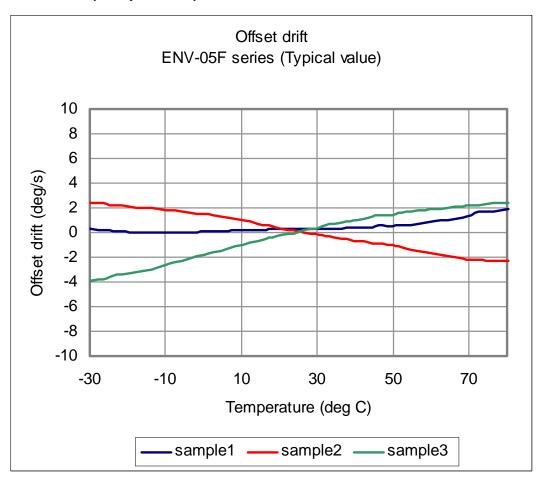
The static output change over operation temperature.
