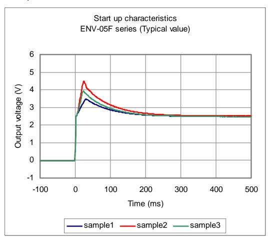
The static output characteristic after the first application of supply voltage.
