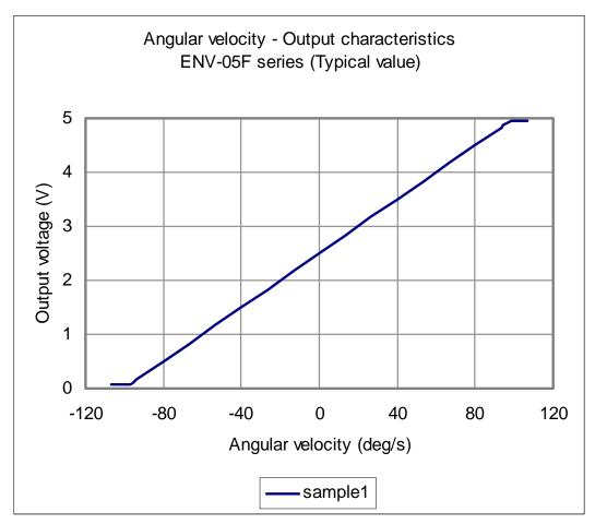
The relationship between output voltage and angular velocity Output voltage is in proportion to angular velocity.
