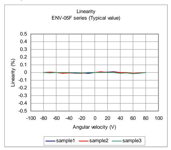
The linearity of output voltage with angular velocity
