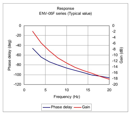
The phase delay with input angular velocity
