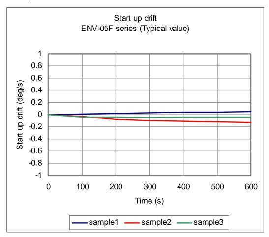
The static output change for 10 minute period beginning ten seconds from the first application of supply voltage.
