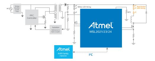
This diagram depicts a typical application using the Atmel MSL2021/23/24 LED drivers, which support the widest power levels.
