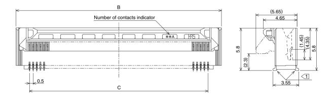
Note 1: The coplanarity of each terminal lead within specified dimension is 0.1 mm Max.
