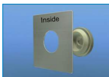
Push the grommet into the hole.
