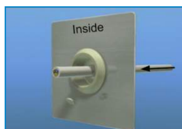
Pierce the grommet with the cable.
