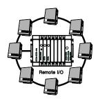
The DXp-40 is also available with the Allen Bradley Remote I/O interface technology, which provides a very simple way to communicate weight and diagnostics information to the PLC-5 series of programmable logic controllers. Also, the DXp-40 can communicate using MODBUS™ or other industry standard protocols.
