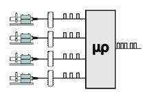
A patented method to control the timing of several dependent A-D converters with a single microprocessor allows for the use of individual transducer data without accumulated errors due to mass moving within a vessel. This capability makes it possible to individually digitize each transducer in a multi-cell system and achieve the benefits of additive resolution and system redundancy.
