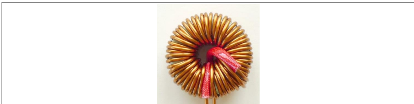
Figure 4 Photograph of PFC choke
