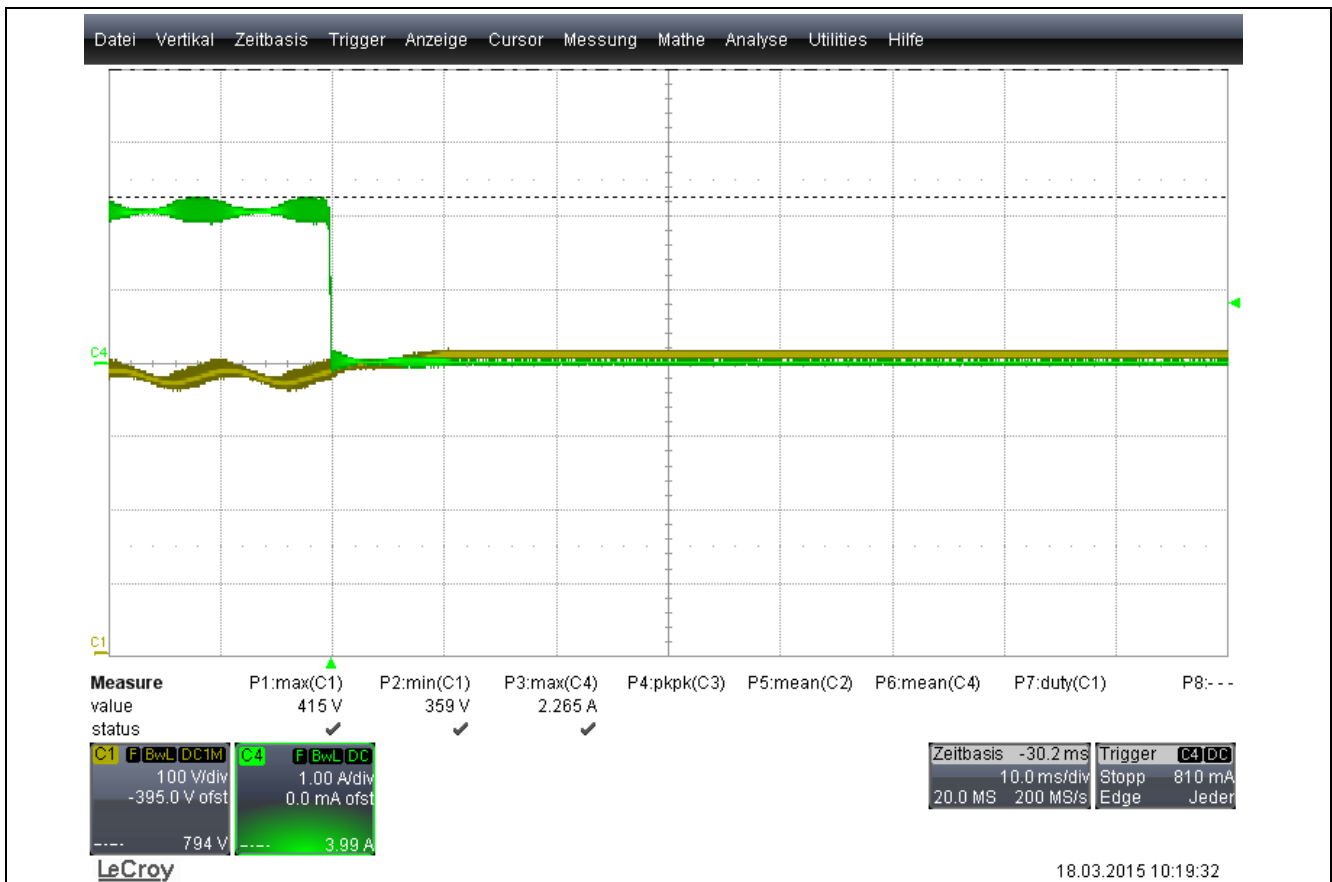
Figure 19 Load step 100% of load → 0% of load V_{in}=90 V_{AC}
