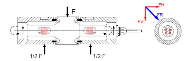
The reactive force FR on the roller or on the KISD-6 load cell will consist of three basic forces:
