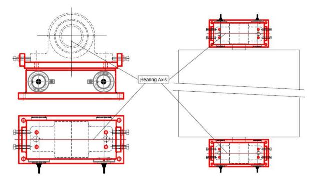
Adjusting the parallelism of the measurement roll relative to the other rollers of the machine. This can be done manually, or if requested at order, the FMU-5 tensiometers can be delivered with screw adjustments on each side of the top plate, to simplify this operation.
