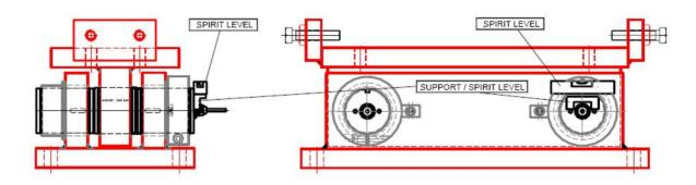
Depending on the application, the wrap angels and the nominal tension forces, the KISD-6 load cells can be orientated either vertically, horizontally or in the direction of the resultant force FR. In order to have the KISD-6 load cells properly orientated, check the arrow direction.
