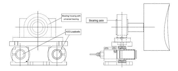
Other basic principles are used for the FMU-1 tensiometers:
