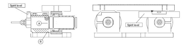
Depending on the application, the wrap angels and the nominal tension forces, the KIS load cells can be orientated either vertically, horizontally or in the direction of the resultant force FR. In order to have the KIS load cells properly orientated, check the arrow direction.
