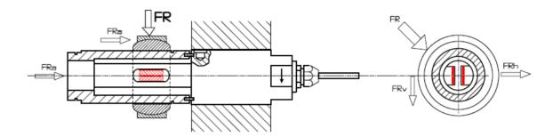
The reactive force FR on the roller or on the KIS load cell will consist of three basic forces:
