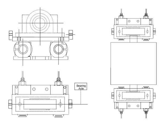
Adjusting the parallelism of the measurement roll relative to the other rollers of the machine. This can be done manually, or if requested at order, the FMU-1 tensiometers can be delivered with screw adjustments on each side of the top plate, to simplify this operation.
