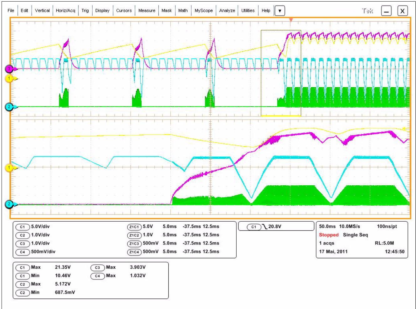
Figure 24 RUN Mode Restart from Short OUT
